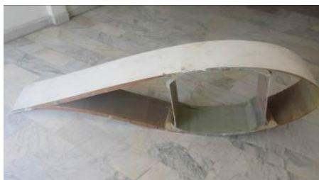
Fig. 2 Cross section view of blade spar
