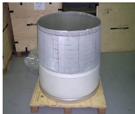
Fig. 5 Root joint of current blade
